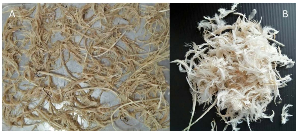
Fig 1 The preparation of chicken feathers prior to the alkaline hydrolysis: (A) chicken feathers after cleaning, (B) defatted chicken feathers.
