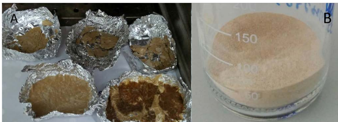
Fig 3 The solubilized keratins were recovered by ammonium sulfate precipitation: (A) crude keratins were dried in hot oven until the constant weight was reached, (B) the end product after an extraction process.
