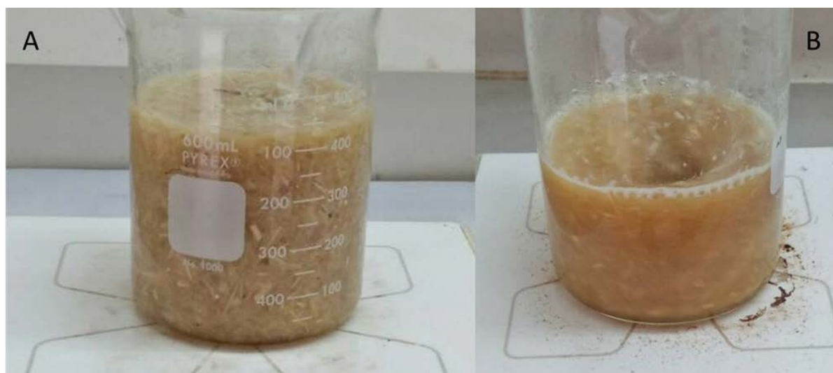
Fig 2 Keratin extraction via alkaline hydrolysis: (A) feathers were mixed with 2.5% NaOH solution (pH 13) and equipped on hot plate, (B): feathers were constantly solubilized over time.
