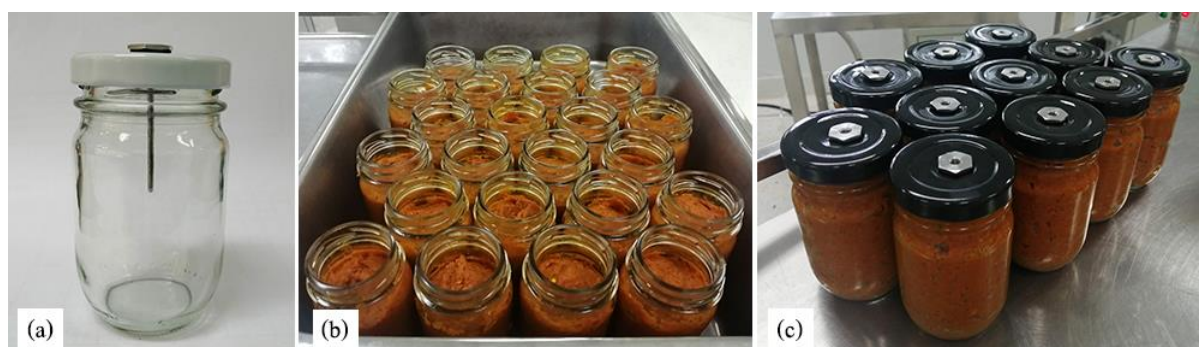
Figure 1 An empty glass bottle and thermocouple sleeve installed through the lid (a), the weighted 100g samples of KS curry paste filled in glass bottles (b), and the hermetic seals made under vacuum to cover samples for sterilization (c). The cases GC, PP and MM were quite similar in appearance.
