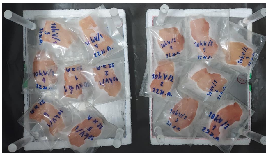
Fig 2 Arrangement of chicken breasts, with 2 cm. thickness and weighted for 38 \pm 2 g in LDPE vacuum bag, on electrode.
