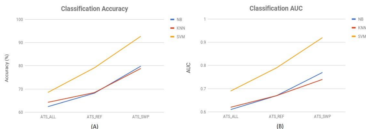
Figure 2 Classification results of NBC, KNN and SVM with attribute selection cases (ATS_ALL, ATS_REF, ATS_SWP) for accuracy (A) and AUC (B).
