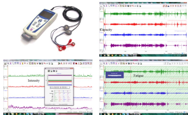
Figure 2 EMG device and samples of the graphic user interface from Megawin software, Finland, used for assessment.
