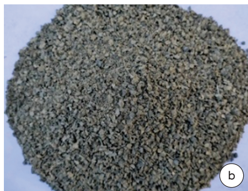
Figure 1 Salt farming residual (Kee dad na kluer) before (a) and after (b) grinding
