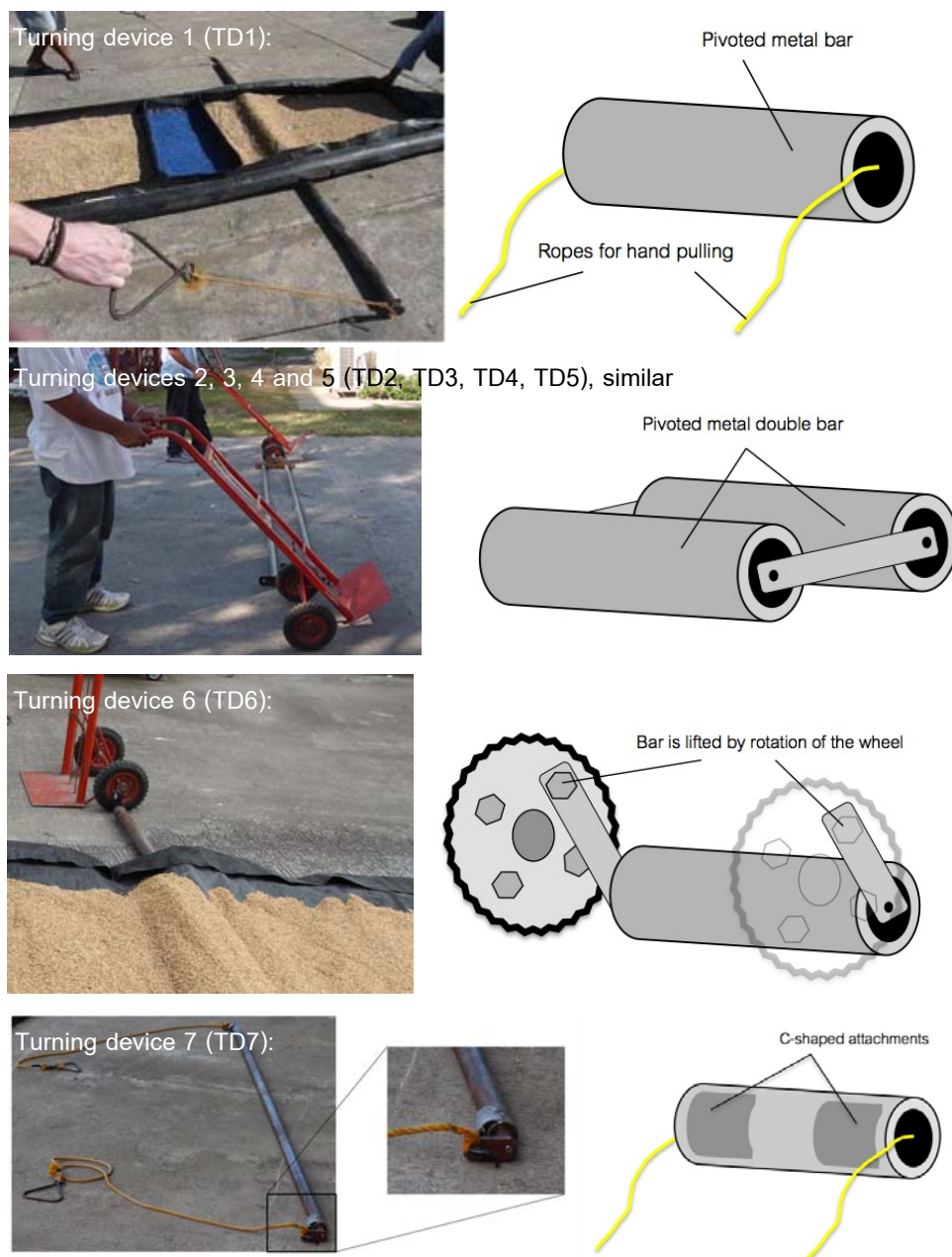
Figure 2 Turning Device 1 enabled paddy rice turning via hand pulling by two people. The device consisted of a single metal bar with a diameter of 5 cm. Turning devices 2, 3, 4, and 5 were operated via a dolly. TD2 incorporated a double bar at diameters of 2.5 cm each, whereas TD3 used two bars with 5 cm diameter. Both TD4 and TD5 induced horizontal oscillation and were operated with double bar (diameter = 2.5 cm) and single bar (diameter = 5 cm), respectively. Turning device 6 consisted of a single metal bar (diameter = 5 cm) operated via a dolly with the bar attached to the outer rim of the wheels in order to create up-and-down motion (vertical oscillation) in the bulk. Turning device 7 used a hand-pulled single bar (diameter = 5 cm) with C-shaped attachments welded to the bar in order to create vertical oscillation.
