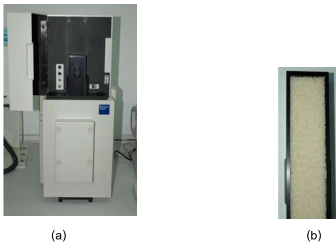
Figure 1 Equipment for NIR spectral acquisition of milled rice (KDML105).
