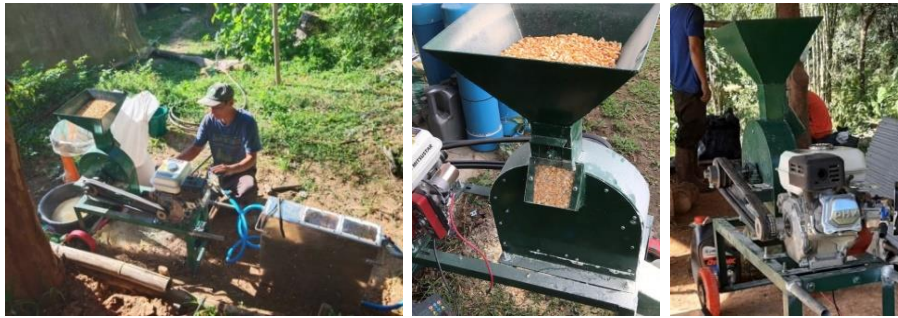
Figure 2. Using biogas to supply small engine (6.5 hp) for grinding corn grain at highland farm
