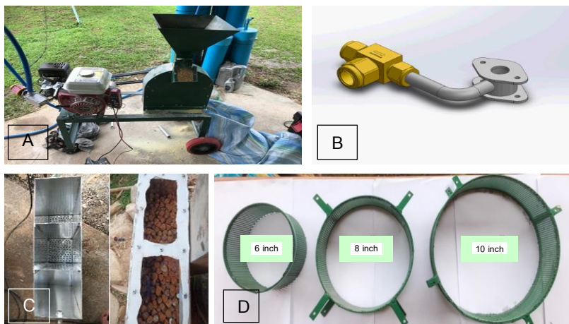
Figure 1. Biogas small engine 6.5 hp (A), mixer (B), hydrogen sulfide ( H_2S ) filter (C), grinding head size of hammer mill (D)
