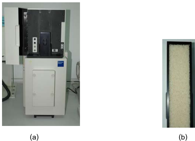
Figure 1 Equipment for NIR spectral acquisition of milled rice (KDML105).
