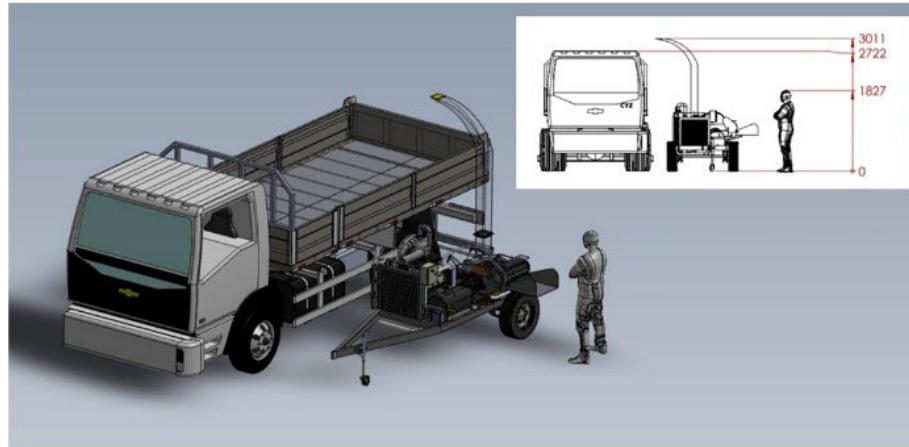
Figure 3 Characteristics of sending shredded wood chips to 6-wheel trucks
