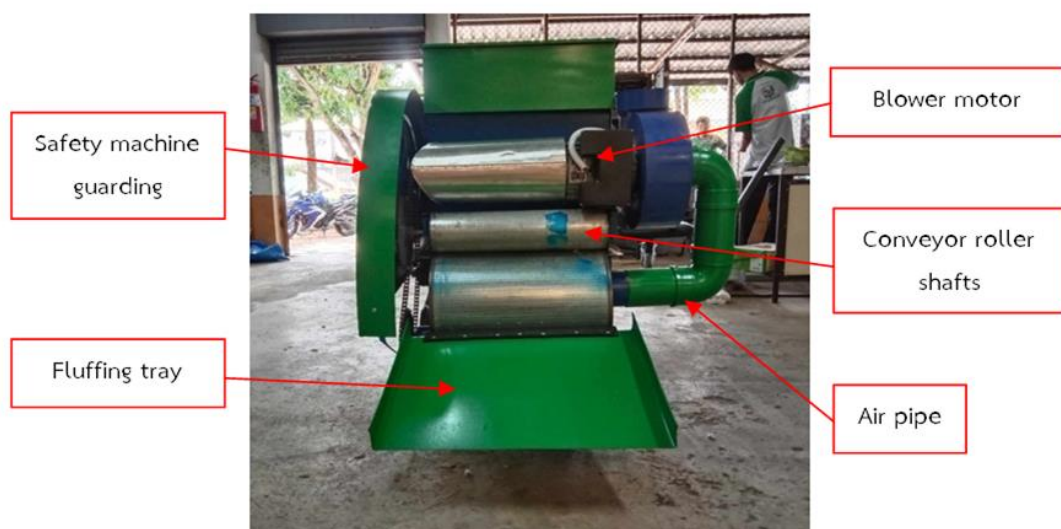
Figure 7 Rear components of a machine for a cotton fiber preparation machine
