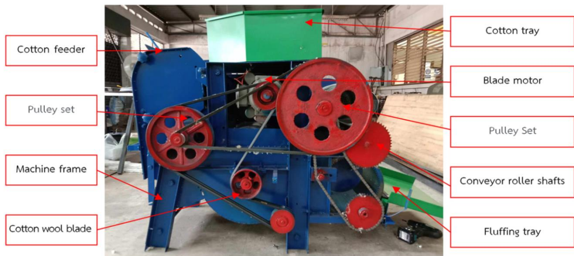
Figure 4 Side components of a machine for a cotton fiber preparation machine
