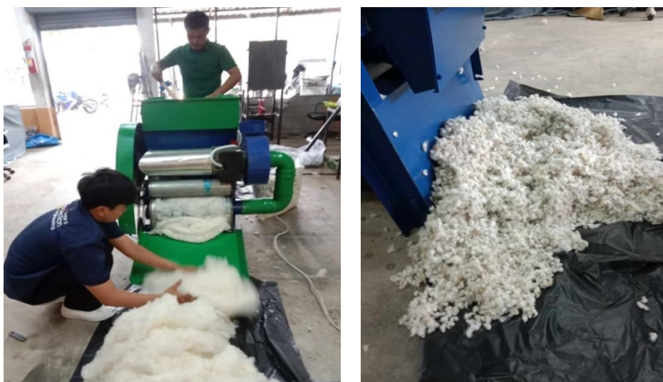
Figure 10 separate the seeds and fluffing cotton wool and cotton seeds with impurities
