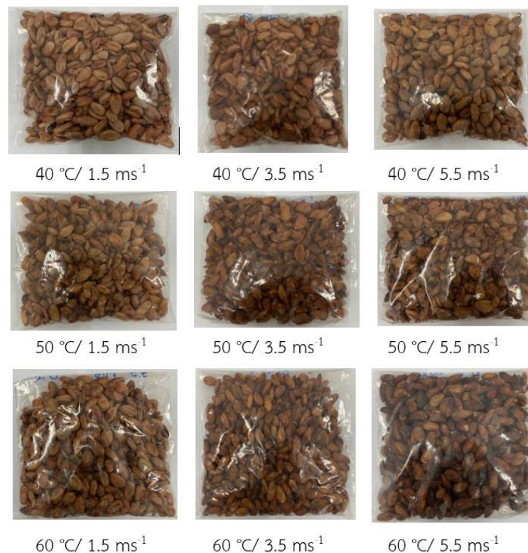
Figure 10 Comparison of cocoa bean color at temperatures of 40, 50, and 60 °C with air velocities of 1.5, 3.5, and 5.5 m/s.
