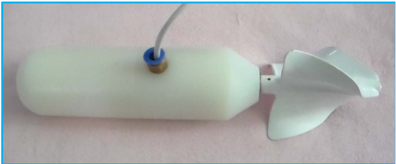
Fig.5 Assembled flow meter
