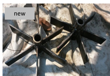
d) Iron driving shaft
