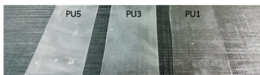
Figure 7 The appearance of the PU films with 2:1 ratio of NCO:OH with showing an increasing of the opacity with the amount of BHET.
