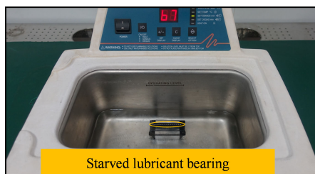
Figure 11 Removal of lubricants from the linear bearing.
