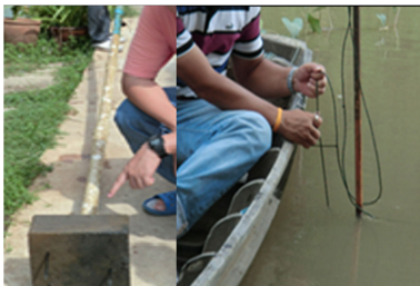
Figure 3 Water level pole and plumb for measuring water level.
