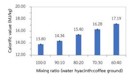
Figure 4 Calorific value of fuel pellets produced from water hyacinth mixed with coffee grounds at different mixing ratio.
