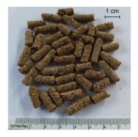
Figure 3 Pellets produced from water hyacinth and coffee grounds (60:40).
