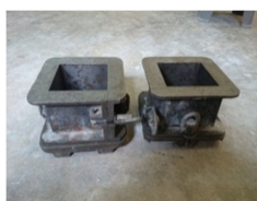
Figure 2 Steel square shape mold size 10×10×10 cm.
