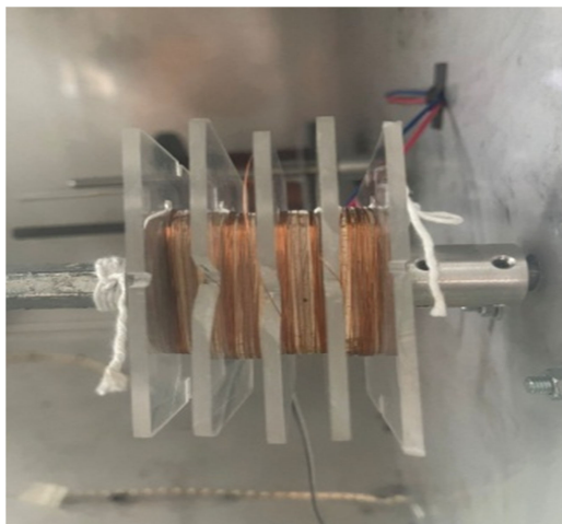
Figure 12 Coils wound with automatic winding machine.
