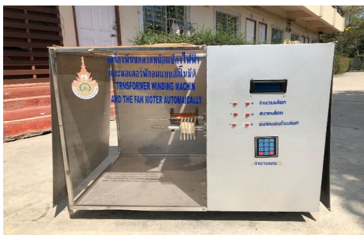
Figure 4 An automatic winding machine for transformers and fan motors.
