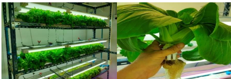
Figure 12 Lettuce growing under white light-emitting diode light and 240 g Cantonese lettuce under the artificial light plant factory by Watjanatepin, & Srichanin (2021).
