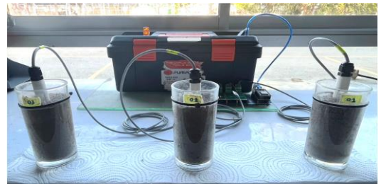
Figure 4 Measurement of soil moisture using soil stick sensors.
