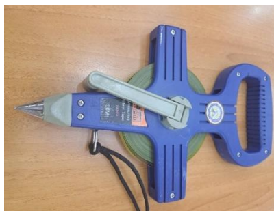
Figure 2 Measuring tape 50 meters certified by Central Office of Weights and Measures.
