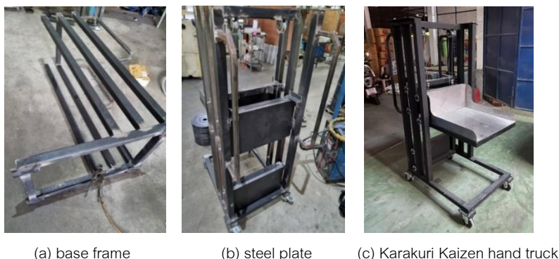
Figure 4 Karakuri Kaizen hand truck building.
