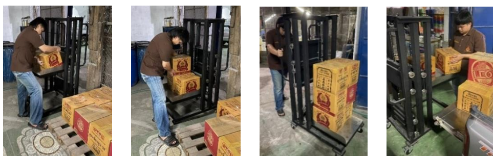
Figure 5 Karakuri Kaizen hand truck process (after improvement).
