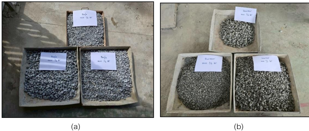
Figure 2 (a) Coarse aggregate of limestone, and (b) coarse aggregate of basalt.
