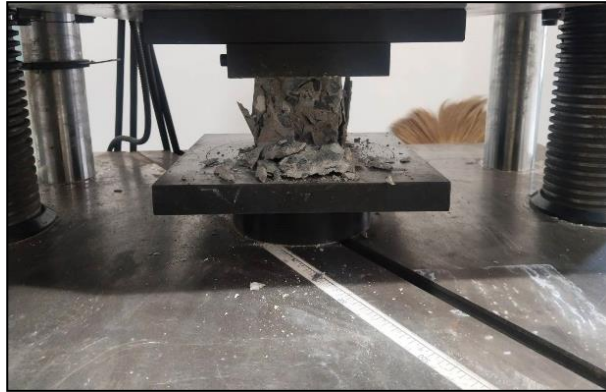
Figure 6 Compressive strength test of concrete.
