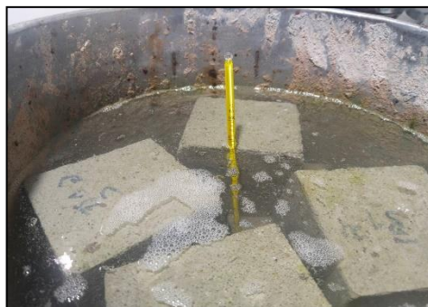
Figure 5 Concrete curing under specified conditions.
