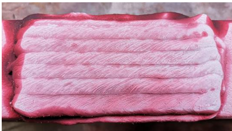
Figure 5 Weld inspection using penetrant testing (PT).
