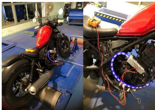
Figure 1 Experimental setup and instrumentation of the motorcycle using a dynamometer.
