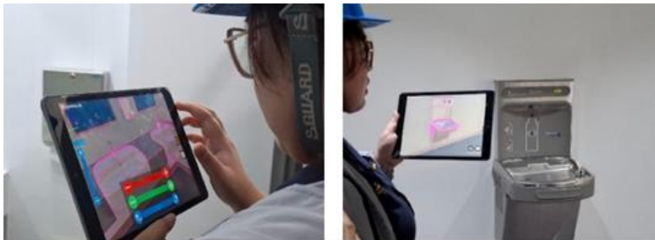
Figure 2 On-site AR inspection workflow using a tablet device with the Gamma AR application: loading the selected BIM model, aligning coordinates with the actual space (left), and capturing paired images of the AR overlay and actual installation for verification (right).
