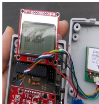
Figure 14 Nokia 5110 LCD display
