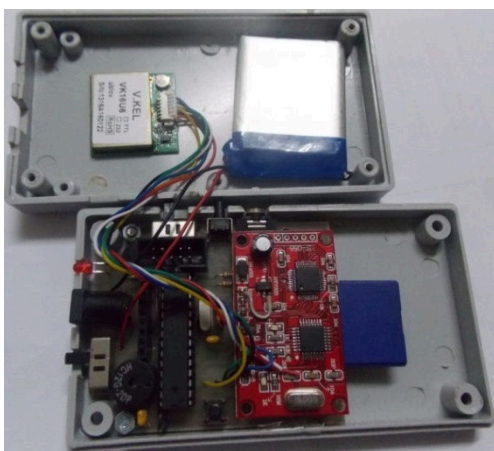
Figure 9 Inside Bus stop Announcement box
