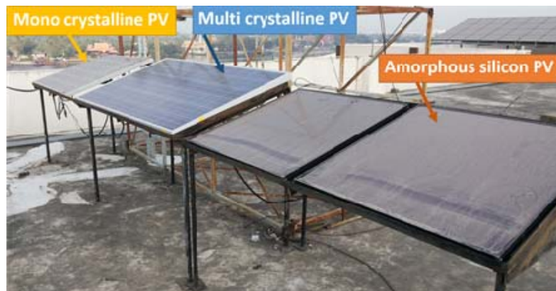
Figure 2 The installation of the three types of PV set up for the experiment
