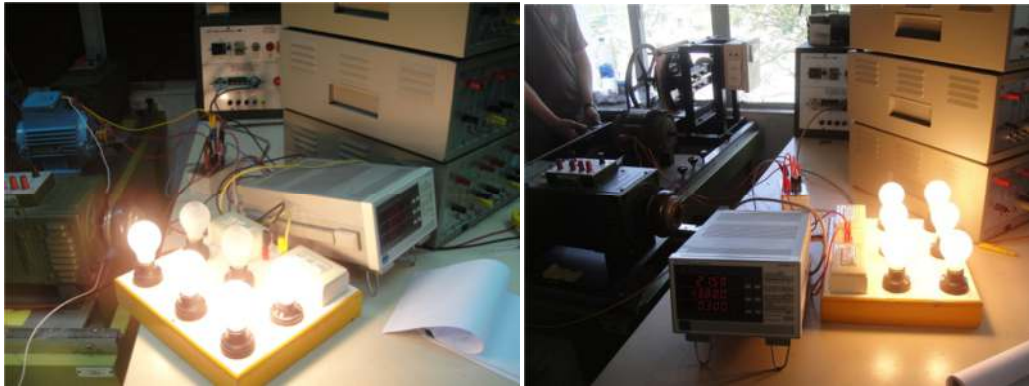
Figure 6 Testing of the low speed generator with the AC-load.
