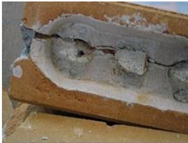
Figure 7 Concave appearance under the interlocking blocks from Chiang Mai, Saraburi, and Chantaburi.
