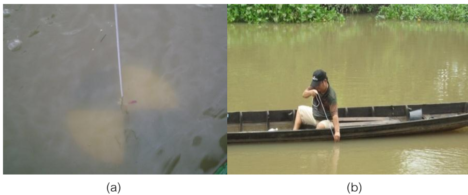
Figure 4 The procedure of collection, the secchi disc.
