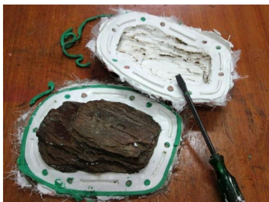
Figure 3 Sedimentary rock that brought to make two sid rubber molds which were covered with fiber glass.
