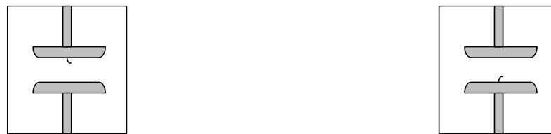
a) Corona discharge at high voltage side in air b) Corona discharge at low voltage side in air
