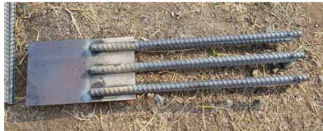
Figure 1 Deformed bars welded to steel plate, used in the experimental investigation.
