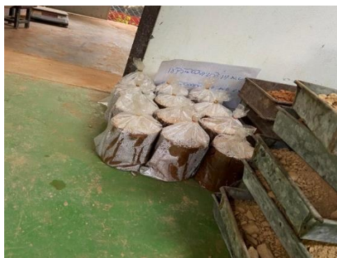
Figure 4 Lateritic soil improved with cement curing in closed plastic bag
