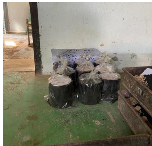
Figure 5 Lateritic soil improved with cement and POFA curing in closed plastic bag
