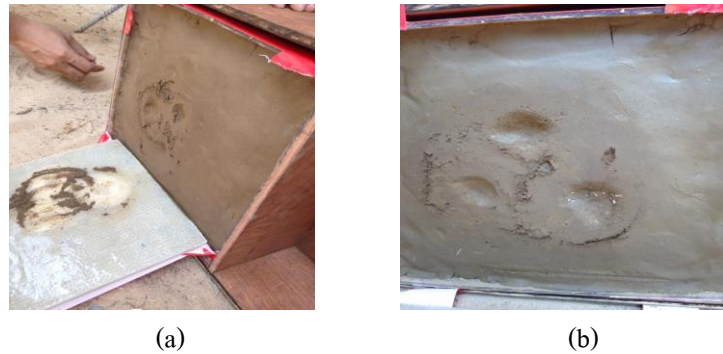
Figure 9 Indentations of backing materials behind 30-layers armor plates after hit by .357 Magnum FMJ bullets (a) 0-degree alignment (b) 45-degree alignment
