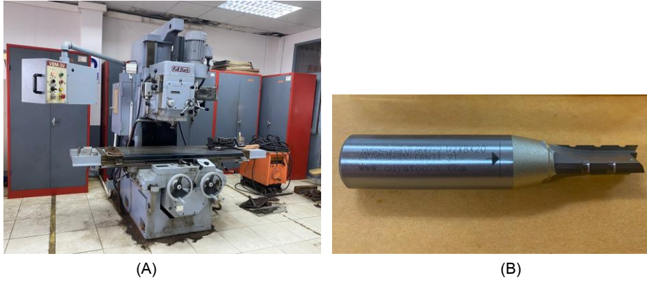
Figure 2 (A) a vertical milling machine and (B) an end mill.
