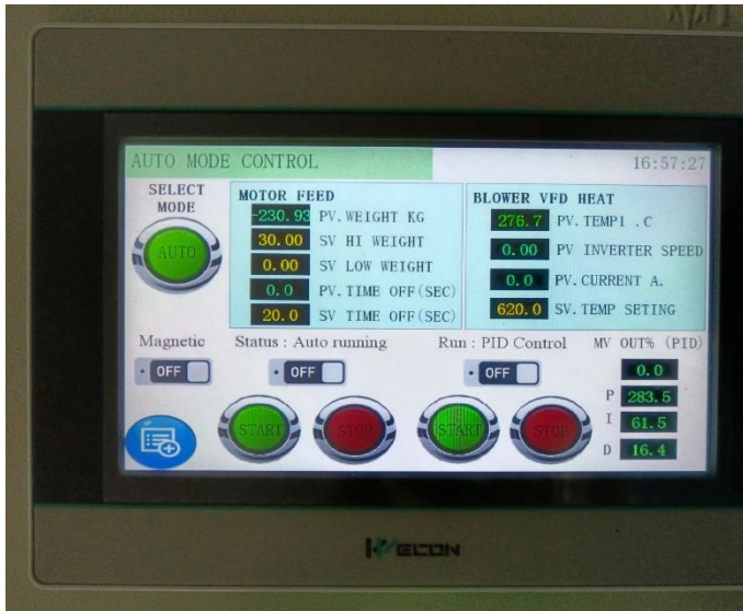
Figure 5 Operation screen in AUTO mode
