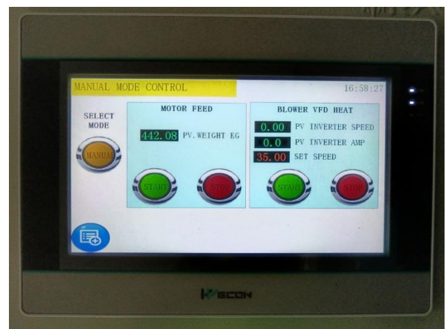
Figure 4 Operation screen in Manual mode
