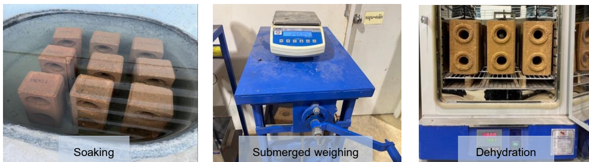
Figure 4 Evaluation of water absorption capacity of interlocking blocks.
