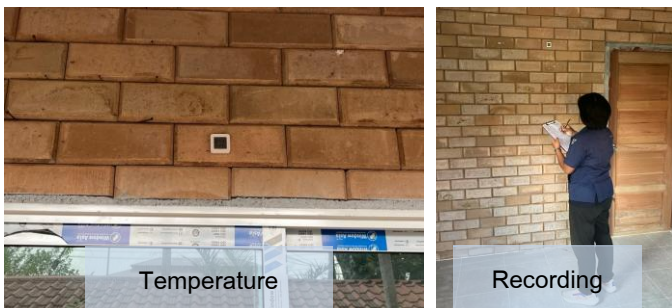
Figure 11 Temperature recording of a house built with interlocking blocks containing para-wood ash.
