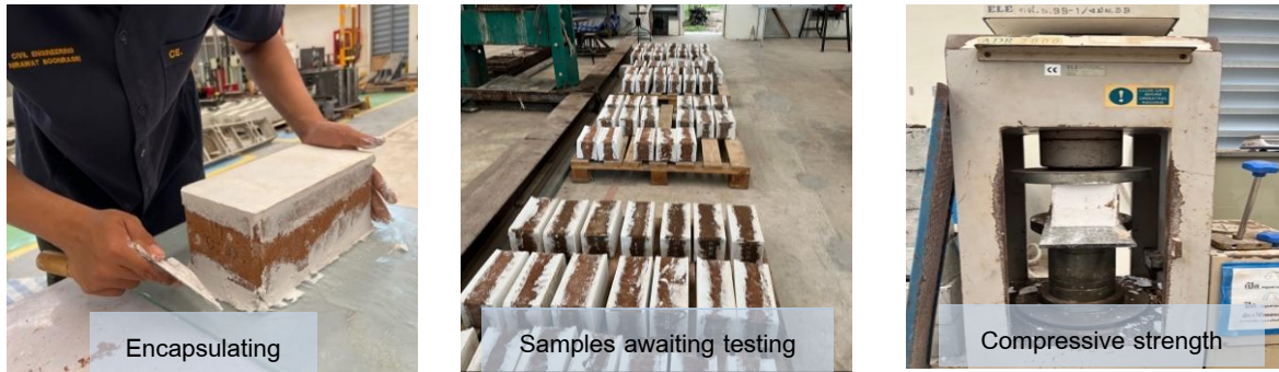
Figure 3 The compressive strength test of interlocking blocks.
