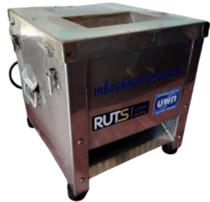
Figure 10 The Constructed Dried Fish Strip-Cutting Machine
