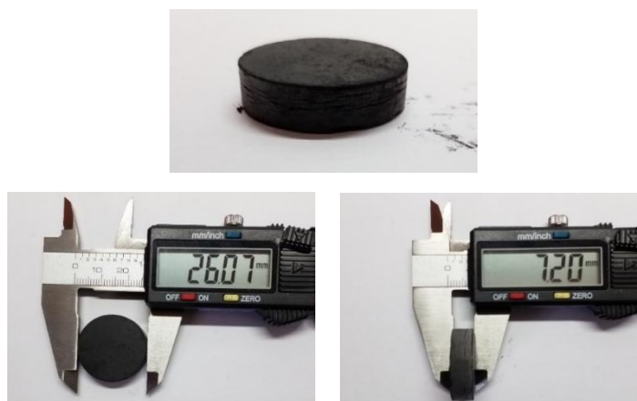
Figure 4 Appearance and dimensions of a sintered membrane.
