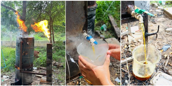
Figure 2 Community-scale fixed-bed pyrolysis reactor (left) with pyrolytic oil collection at the condensate outlet (center and right).
