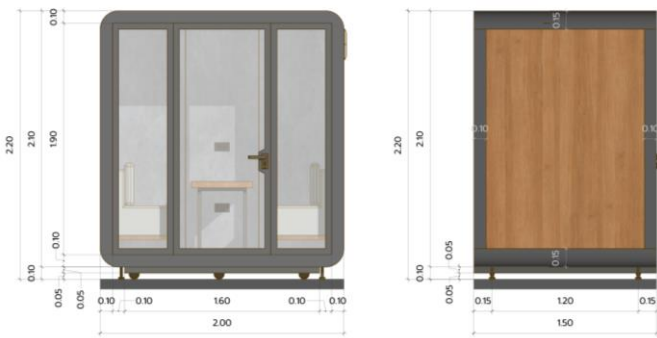
Figure 2 Schematic design and full-scale prototype of the modular acoustic pod used for field sound insulation evaluation.
