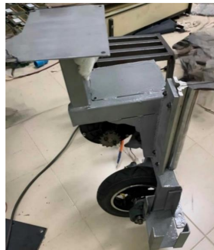
Figure 3 The e-tugger's main structure for installing other components
