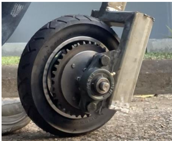
Figure 4 A rear pneumatic wheel, installed on the fork of the e-tugger structure
