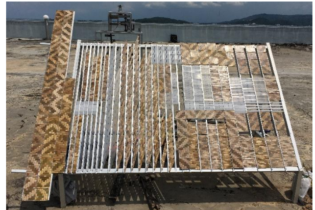
Figure 3 Experimental set-up for sandwich composites between plastics and weaving bamboo plates under natural weathering test.
